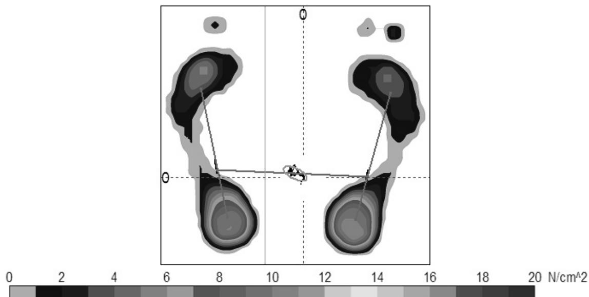
Fig. 4. Distribution of foot pressing forces in the standing position (www.zebris.de)
